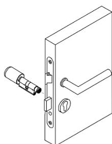
Figure 1: Installing the cylinder
