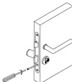
Figure 2: Fixing the cylinder
