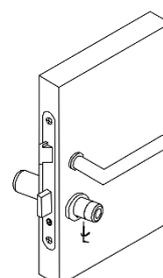
Figure 3: Attaching the knob
