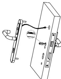
Figure 2: Connecting the cover on the outside
