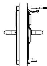
Figure 3: Screwing the electronic handle
